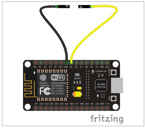
Figure 8-2. Simple sensing with two wires
