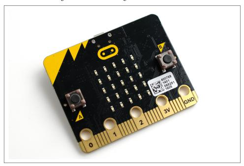
Figure 3-2. The front of the BBC micro:bit
