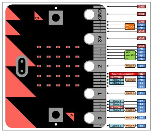
Figure 9-3. The micro:bit's pinout diagram
