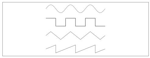
Figure 11-1. The shapes of four waveforms to change the timbre of the output. From the top: sine, square, triangle, and sawtooth.
