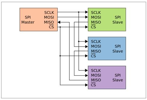
Figure 9-5. SPI configuration with three daisy-chained slaves
