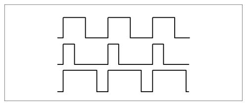
Figure 7-1. Three different PWM signals.
