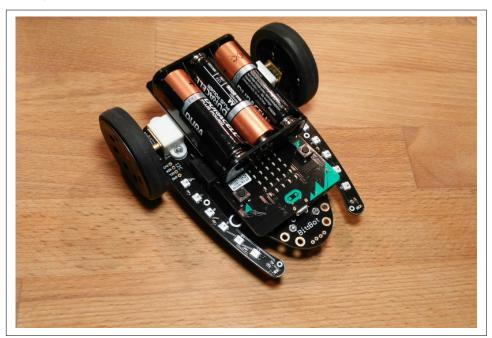
Figure 12-5. The Bit:Bot by 4tronix
