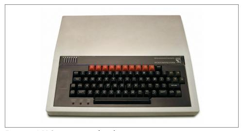
Figure 3-1. A BBC microcomputer from the 1980s
