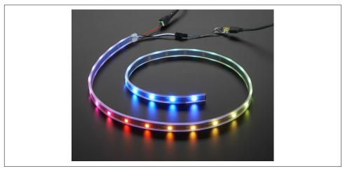
Figure 7-2. A strip of NeoPixels. Also available as rings, flexible boards, and sticks.
