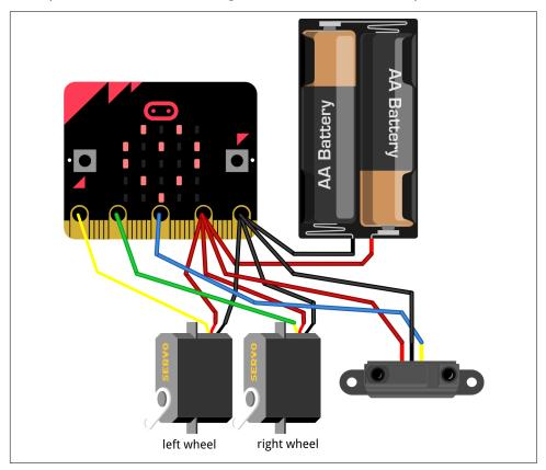
Figure 12-4. The trundlebot wiring diagram
