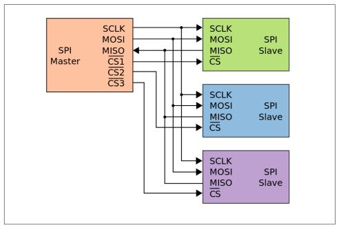
Figure 9-4. SPI configuration with three independent slaves
