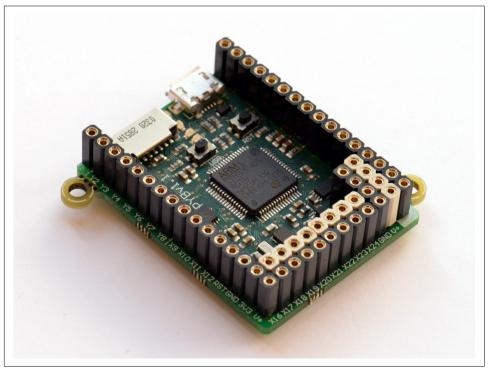
Figure 2-1. The original PyBoard is about the size of a large postage stamp
