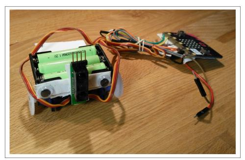
Figure 12-2. The trundlebot showing an improvised chassis held together by stickybacked plastic, twisted wires, tape, and a rubber band
