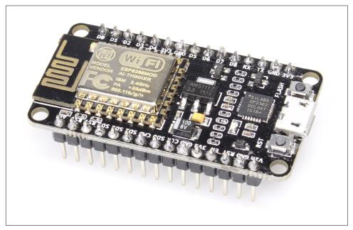
Figure 5-1. A typical ESP8266-based board
